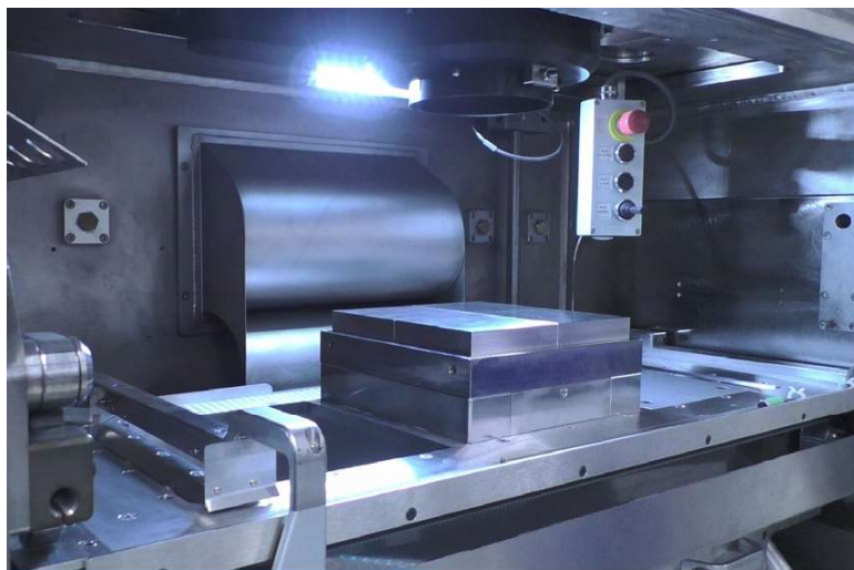
Fig. 1 An AMcarrier and BuildPals inside a DMP Flex 350 PBF-LB machine (Courtesy System 3R)
