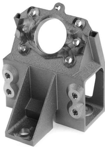
Fig. 5 An aerospace satellite bracket case study developed with 3D Systems utilising the System 3R system. Top: parts arranged on individual BuildPal build plates; middle: a part on a BuildPal before machining (left) and after (right); Bottom: the finished part removed from the build plate (Courtesy System 3R)
